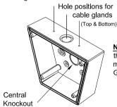
NOTE: Ensure that the IP integrity is maintained during Gland Fitting.
